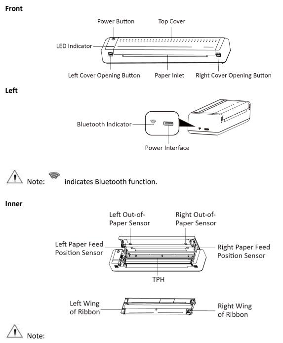
Out-of-paper sensor and paper feed position sensor:
