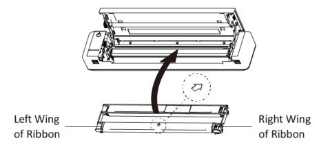
**Note:** To avoid errors when loading the ribbon, please make sure that the arrow direction marked on the ribbon module align to the printer.
